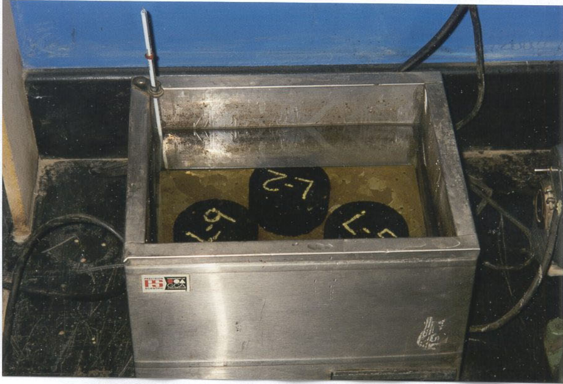
CONDITIONED SPECIMENS IN 60°C WATER BATH (ALL METHODS)
