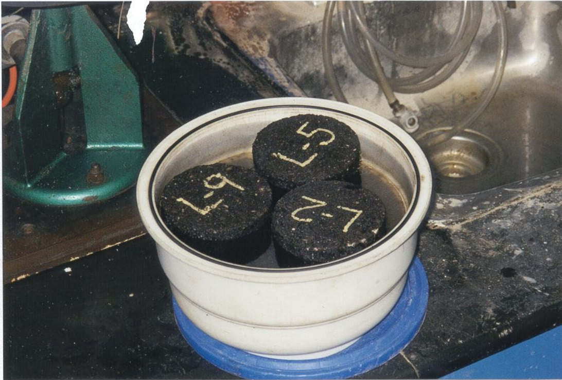
CONDITIONED SPECIMENS PREPARED FOR PARTIAL SATURATION UNDER VACUUM (MTO, ASTM, AND AASHTO METHODS)
