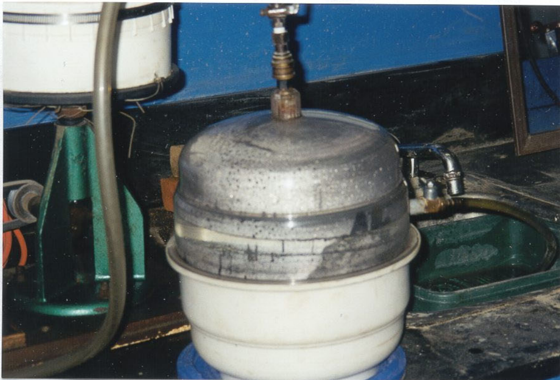
VACUUM SATURATION USING TYPE F PYCNOMETER IN PROGRESS
